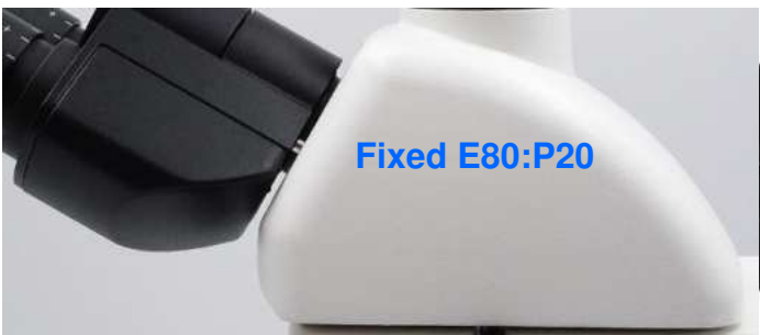
Trinocular Head Light Split Optional Between Switch E100:P0/E0:P100 & Fixed E80:P20 In Fixed Light Split, Eyepiece 80% : Photo 20% User Can View Image At Same Time In Both Path In Switch Light Split, Eyepiece 100%:Photo 0% / Eyepiece 0%:Photo 100%, Camera Can Have 100% Light For Photo Capture.
